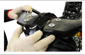
Unscrew and remove the five rear fixing screws.
