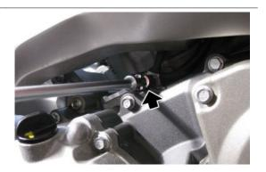
Unscrew and remove the two screws of the ECU.
