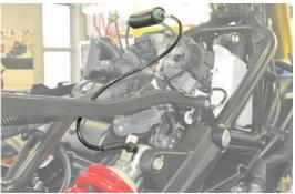
When removing the shock absorber pay attention to the electric motor, it must be removed from the frame taking care not to damage it.
