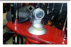
Discharge the spring and remove the suspension from the specific tool
