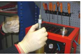
Remove the spring paying attention to drain the oil correctly.
