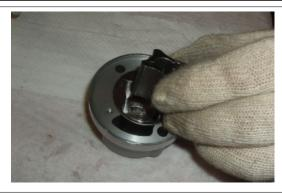
Remove the oil pump stator.
