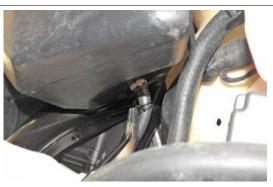
Unscrew and remove the two fixing screws that connect the tank to the underfairing.
