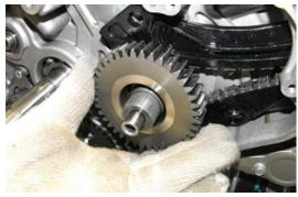
Fit the special tool, tightly fastening the three screws securing the tool onto the crankcase.
