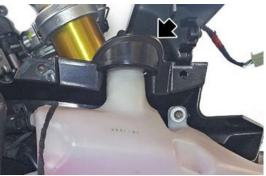
Slide off the sleeve and empty the system completely.
