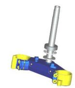
Install the upper bearing on the steering yoke pin as shown in the figure, with the conical part facing downward.
