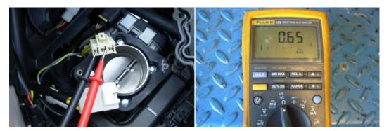
Resistance of the wires read on the display = 0.47 Ohm
