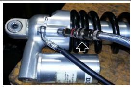
Connect the tube for the oil bleeding/ filling to the tool
