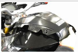
Undo and remove the two mounting fixing screws.
