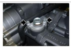
• Insert the spring and tighten the screw together with the washer.
