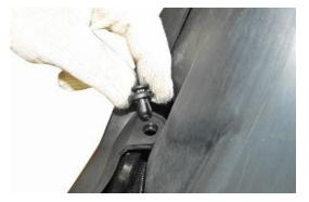
Release the fairing from its fasteners.
