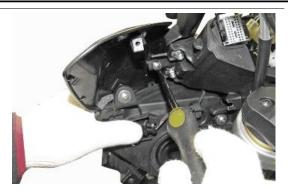
Undo and remove the light unit lower screw.
