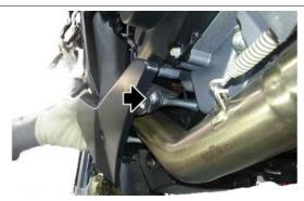
Unscrew and remove the front fairing lug fixing screw.
