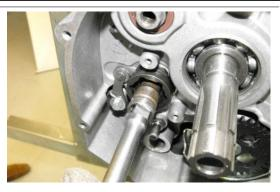
Unscrew and remove the nine flywheel side M8 screws.
