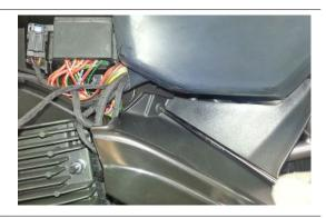
Unscrew and remove the front screw placed near the radiator.
