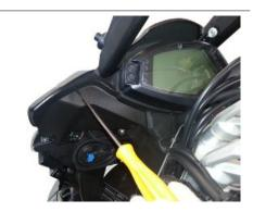
Unscrew and remove the two fixing screws of the central dashboard.
