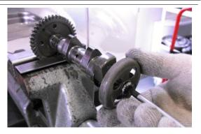
Remove the counterweight and decompression device with the relevant spring.
