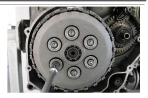
On reassembly, replace the gasket under clutch cover.
