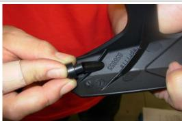
Position and fasten the top screw ensuring to insert the bushing between the hand guard and the handlebar fastening point.
