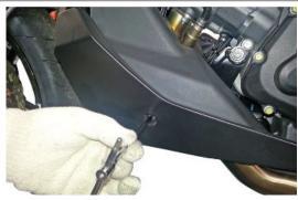
Unscrew and remove the left fairing lug rear fixing screw.
