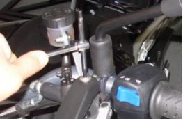
Place the hand guards fastening them on the sides using TCEI M6 X 50 screw being careful when inserting the bushing.
