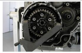
Unscrew and remove the clutch hub nut.
