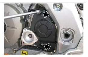
Unscrew and remove the two clutch support screws.
