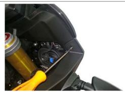
Remove the expansion cap placed on the side part of the fairing, near the turn indicator.
