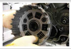
Collect the spacer and the needle bearings.
