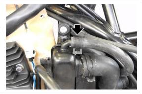
Operating from the right side, unscrew and remove the radiator upper screw.
