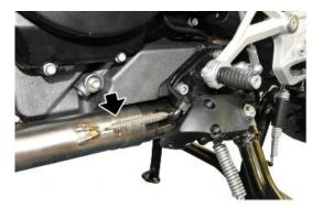
Unscrew and remove the three nuts from the front exhaust manifold
