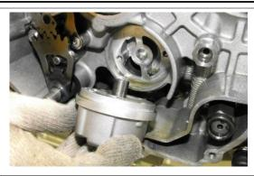
• Fit the protection and tighten the two retaining screws.
