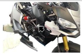
Undo and remove the six fixing screws of the central cover of the tank.
