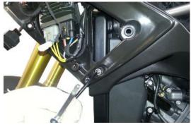
Unscrew and remove the rear screw.
