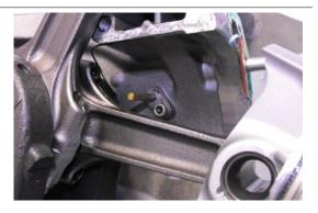
Replace the O-Rings on oil ducts.
