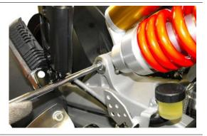
With the specific box-spanner, unscrew and remove the locking ring nut.
