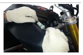
Unscrew and remove the left fairing lug fixing screw.
