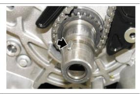
Insert the start-up transmission gear after applying a layer of grease.
