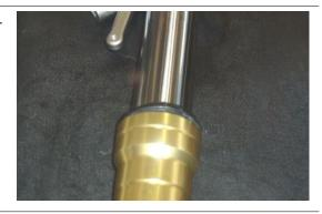
Insert the pumping member pin in the stem.
