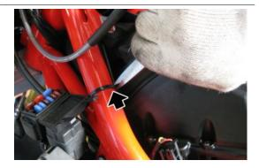
• Disconnect the air temperature sensor.
