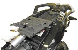
• Disconnect the battery and remove it.
