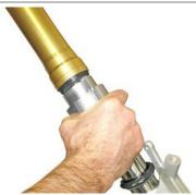
Insert the retainer ring in its position.
