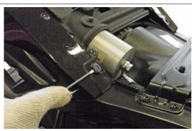
Undo and remove the six fixing screws
