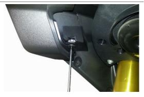
Unscrew and remove the light unit upper fixing screw.
