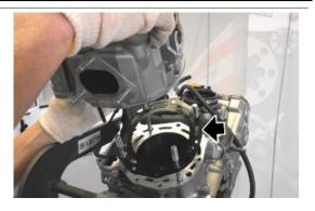
Remove the fixed chain slider.
