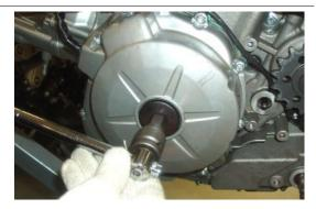
• Unscrew and remove the ten screws.
