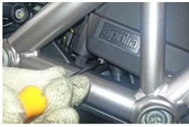
Unscrew and remove the control unit fixing screw.
