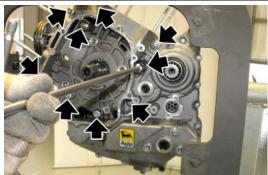
Unscrew and remove the eleven flywheel side M6 screws.
