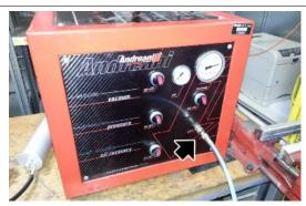
After the bleeding and the oil filling remove the tube from the joints
