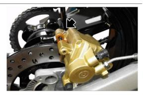
Remove the pin by sliding it backwards.
