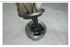
• Collect the lock pin from the shaft.
