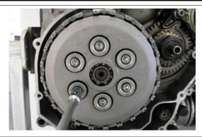
Remove the thrust plate, the plates and belleville washer.
