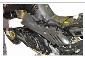
For the left side fairing, the cable of the saddle lock must be removed.
