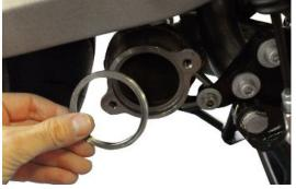
• Remove the catalytic converter.
