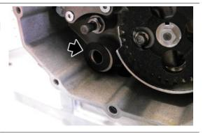
Heat the screws of the gearbox selector mounting plate.
