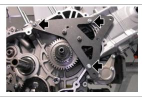
Position the water pump drive gear, the washer and crankshaft fastener nut and tighten it to the specified torque.
