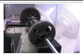
Remove the decompression device housing.
