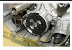
By means of a calliper spanner lock out gear rotation and tighten the retaining nut.
