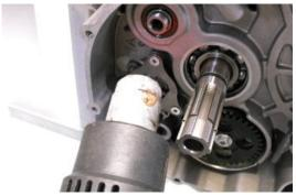
Unscrew and remove the three screws fastening the gearbox selector mounting plate.
