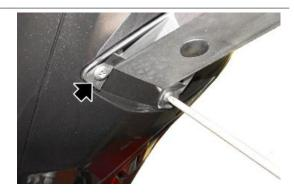
Remove the access cap, unscrew and remove the lower mounting screw.
