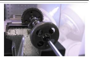
Remove the decompression device housing.
