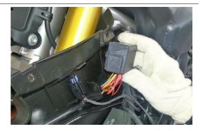
• Cut and remove the clamp.
