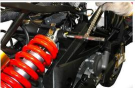
Unscrew and remove the shock absorber lower fixing screw.
