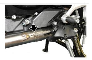
Unscrew and remove the three nuts from the front and rear exhaust manifold
