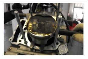
Lock the connecting rod using circlips.
