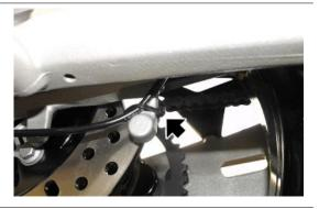
Slide off the rear calliper holding plate, keeping it linked to the brake pipe.
