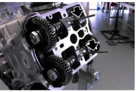
Fit cam tower and tighten the eight screws working in a diagonal sequence and in stages.
