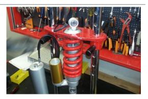
Remove the lock plate of the spring making sure not to damage the cable harness
