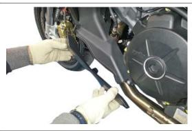
Unscrew and remove the two right fairing lug fixing screws.
