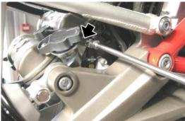
• Slide off the rear top pin and collect the washer.
