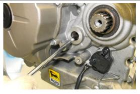
Remove the clutch control rod.
