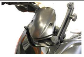
Remove the two screws fastening the lower cover of the dashboard.
