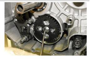
By means of a calliper spanner lock out gear rotation and loosen the nut to remove it.
