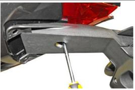
Disconnect the connectors and remove the license plate support.
