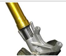
Fit the pumping member inside the stem, paying attention that it is placed inside the seat of the stem.
