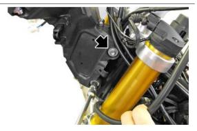
Undo and remove the two shells fixing screws of the instrument support.
