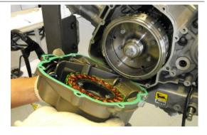
• Collect the gasket and the two dowel pins.
