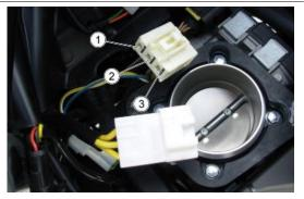
stage "1" (pin 1-2), stage "2" (pin 1-3), stage "3" (pin 2-3).
