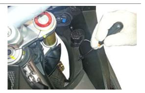
• Undo and remove the front screw.
