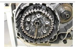
Fasten the clutch housing using the specific tool.
