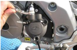
Undo and remove the two screws and remove the pinion protection case.
