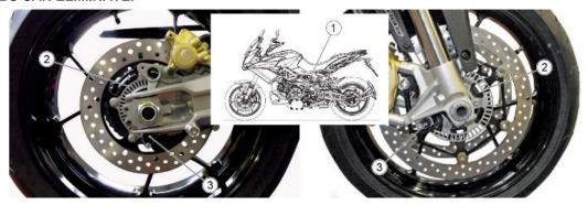
When sensors (3) detect a significant speed difference between the rear and the front wheels (for example, when rearing up on the back wheel), the ABS system could take this as a dangerous situation. In this case, 2 things may occur:
