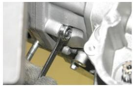
Unscrew and remove the four nuts, proceeding in stages and in a diagonal pattern.
