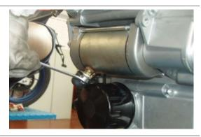
Unscrew and remove the two screws and remove the starter motor.
