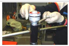
Remove the spring preload pipe.
