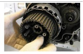
Collect the washer between the clutch hub and the housing.
