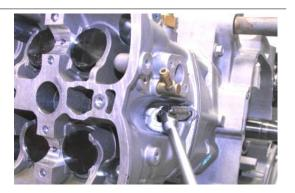
Unscrew and remove the three bottom head fixing nuts.
