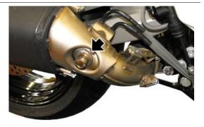
of the valve; the logic and the control of the motor are provided by the VCU control unit (Caponord 1200 Travel Pack) or by the EVC control unit (Caponord 1200).
