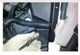
Unscrew and remove the lower fixing screw of the right duct bulkhead.
