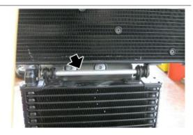
Remove the oil radiator together with support and horn.
