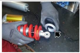
Remove the spring making sure not to damage the cable harness
