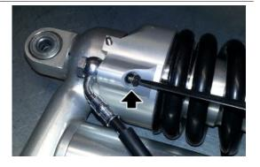
• Insert and tighten the special joint
