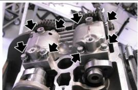
Remove both camshafts, lock them on a vice with aluminium jaws, then tighten the gear retaining nut to the prescribed torque.
