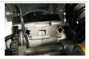
Slide off the rear bottom pin and collect the washer.
