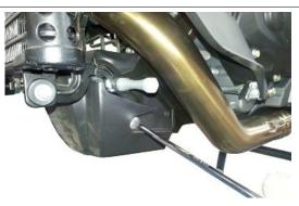
Undo and remove the fixing screw of the oil radiator support.
