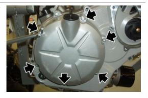
Removing the clutch cover alone is only recommended when replacing the clutch plates. When removing the entire clutch assembly, removing the clutch side cover is recommended.
