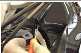
Remove the three expansion caps on the inside of the fairing.
