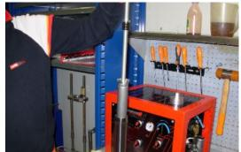
Using a hook spanner lock the pumping member pin and tighten the fixing screw on the fork end to the prescribed torque.
