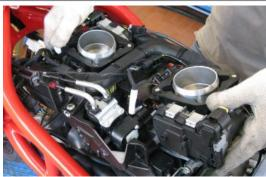
Disconnect the engine temperature sensor from the front cylinder.
