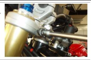
Undo and remove the two screws fixing the instrument panel support to the fork upper plate.
