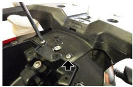
Disconnect the saddle lock by undoing the two screws.
