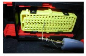
the connector (i.e., all terminals aligned at the same depth) and terminal integrity (i.e., that terminals are not loose, open/bent, etc.). For connectors whose terminals are not visible (e.g. Marelli control unit) use a metal cable of suitable diameter and introduce it carefully in the connector slot at the same depth as for the other terminals of the connector.
