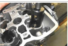
• Remove the cotters using a magnet.
