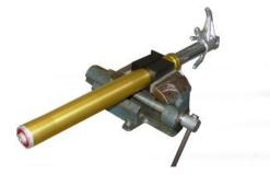
Operating on the upper screw, unload the spring.
