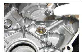
Place the oil seal retainer with its flat side resting against the oil seal.
