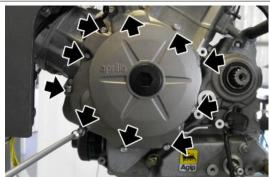
Remove the flywheel cover using the specific tool.
