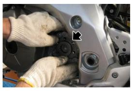
Loosen the screw and slide off the gear transmission connecting rod keeping it linked to the gear shift lever through the rod.
