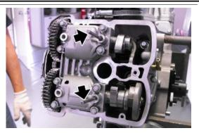
Unscrew and remove the eight fixing screws and remove the cam tower.
