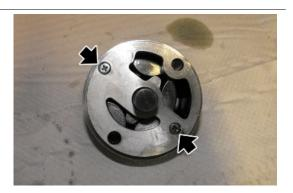
Using a thickness gauge check clearance between rotor and stator and replace the rotor / stator unit if necessary.
