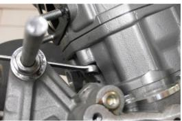
Unscrew and remove the four nuts, proceeding in stages and in a diagonal pattern.
