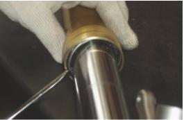
Fit the dust gaiter with the specific tool.
