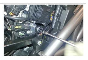
Slide off the control unit from the mountings and remove it from the vehicle.
