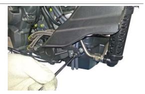
• Remove the right duct bulkhead.
