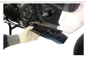
Undo and remove the two upper fixing screws of the right duct bulkhead.
