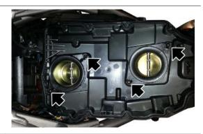
Remove the two intake ducts.
