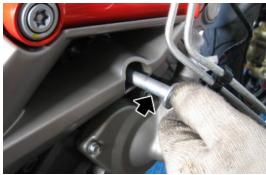
Remove the bottom spacer on the right side.
