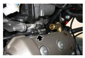
Lift the throttle body but keep it connected to the wiring harness.
