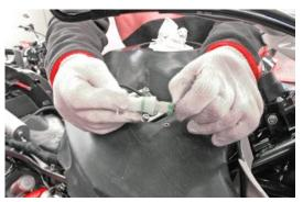
Working from both sides, disconnect both breather pipes.
