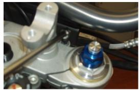
• Slide off the fork upper plate by moving it towards the instrument panel.
