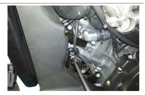
Undo and remove the fairing lug lower screw.
