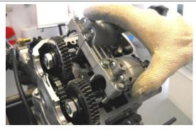
Remove the camshafts with the gears.
