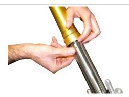
Fit the dust gaiter with the specific tool.
