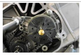
Remove the H2O pump and slide off the drive chain.
