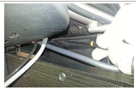
• Separate the two radiators and remove the radiator protection.
