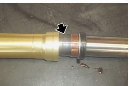
Fit the sleeve on the stem and set the oil seal into position with the aid of the specific tool.
