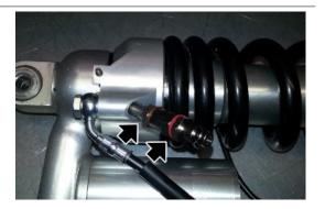
Connect the tube for the oil bleeding/ filling to the joint
