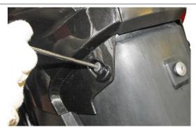
Unscrew and remove the front fixing screw.
