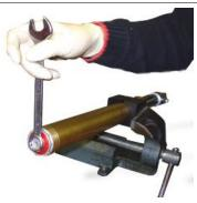
Loosen the cover without unscrewing it completely, using the suitable equipment.
