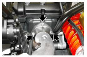
Disengage the spring joining the rear exhaust manifold and the catalytic converter.
