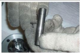
Remove the oil pump rotor.
