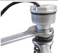
Using a wrench and the special tool, tighten the cap and the ring nut to the prescribed torque.
