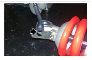
After removing the two fastening screws of the support bracket, remove it
