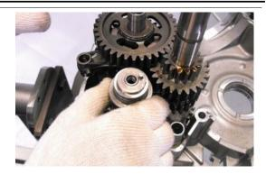
Remove the three gear selection forks.
