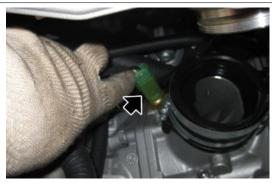
• Disconnect the alternator connectors.
