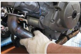
Unscrew and remove the catalytic converter mounting screw
