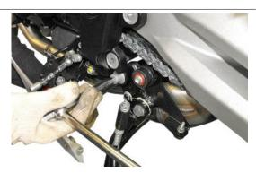
Working on the left inside, unscrew and remove the central stand fixing screw.
