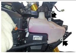
Lower radiator and disconnect the right electric fan.
