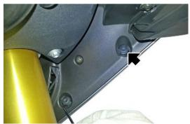
Remove the internal upper expansion cap.
