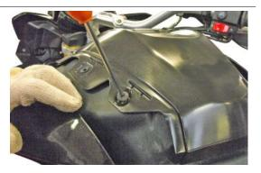
Unscrew and remove the four fixing screws of the tank cap.
