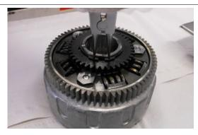
Remove the oil pump control gear.
