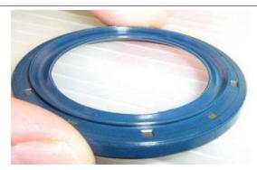
Pass with a brush on the seal ring to lay down potential grease storage.
