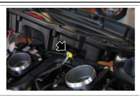
Remove the two clamps from the blowby system.
