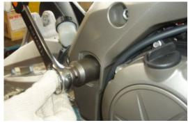
Working from the left side, unscrew and remove the nut and collect the washer.
