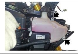
Unscrew and remove the screw indicated in the figure.
