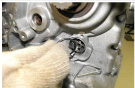
Position the gear sensor and screw the two fixing screws.
