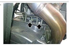
• Undo the radiator fixing screw.
