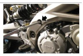
Remove the two spacers. The thinner spacer is on the right.
