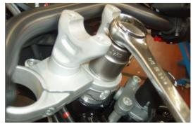
Operating from both sides, loosen the screws fixing the stanchions to the upper plate.
