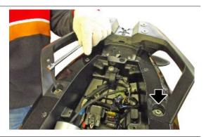
Unscrew and remove the two central fixing screws.
