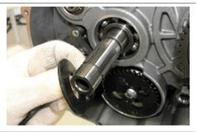
• Fit the needle bearing and the spacer.
