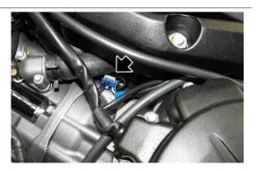
Disconnect the gear in neutral sensor connector.
