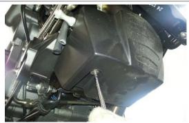
Undo the two upper fixing screws of the fairing lug.
