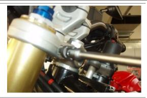
When refitting the U-bolt, position the two references facing the front part of the vehicle.
