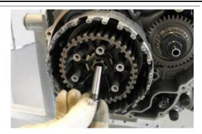
Working on the flywheel side, push the clutch control rod so that it comes out on the other side.
