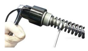
• Before removing the cap (1) from the pumping member, the electric cable harness must be released. To do this, loosen the ring nut (2) and remove the sleeve (3) by unscrewing it.
