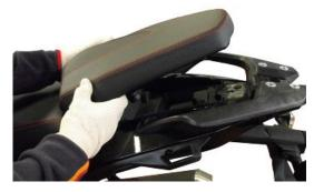
Unscrew and remove the front saddle fixing screw.
